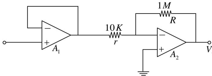
If the input ac signal source has an impedance of  $50k\Omega$ , which of the following statements is true?
