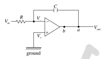
The modification in the circuit required to introduce a dc feedback is to add a resistor
