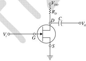
If the drain D - source S saturation current  $I_{DSS}$  is  $10 \, mA$  and the pinch-off voltage  $V_P$  is -8V, then the voltage across points D and S is
