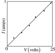
If the error in the slope is  $1.255 \times 10^{-3} \,\Omega^{-1}$ , then the value of resistance estimated from the graph is
