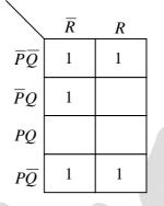
Q.59 The minimized logic expression for the above map is (a)  $Y = \overline{PR} + \overline{Q}$  (b)  $Y = \overline{Q} \cdot PR$  (c)  $Y = \overline{Q} + PR$  (d)  $Y = Q \cdot \overline{PR}$
