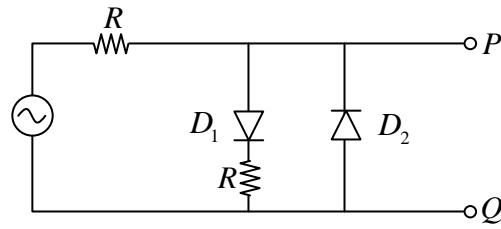
During positive half cycle  $D_1$  is forward bias, when input is less positive than  $+0.7V$ , diode is OFF and output is equal to input. When input is more positive than  $+0.7V$ ,  $D_1$  is ON and output is  $(0.7 + IR)V$ .
