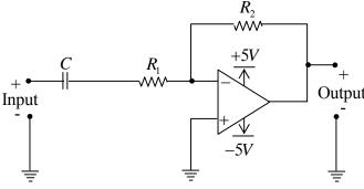
(a) Low pass filter with  $f_{3dB} = \frac{1}{(R_1 + R_2)C} rad/s$
